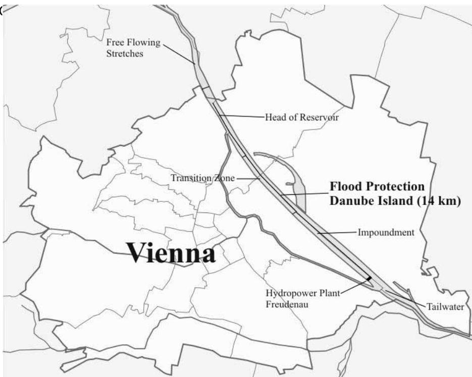
**Figure 1.** Map of the five sections Tailwater, Impoundment, Transition Zone, Head of Reservoir and Free Flowing Stretches in the study area hydropower plant Freudenu, Vienna, Austria.
