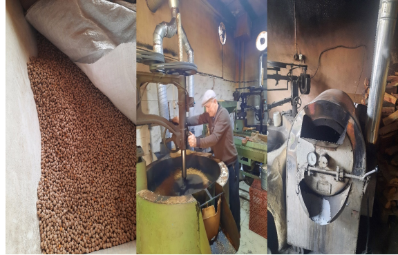
Pic. 2. Fermented Chickpea, Shell Removal Process and Roasting-Speckling Process
